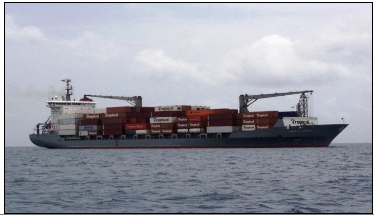
Box 4. Tropical Shipping handles all shipments of cocoa and nutmeg to destinations in the U.S. and Canada. This photo shows a typical container vessel equipped with two container cranes for loading & unloading.
